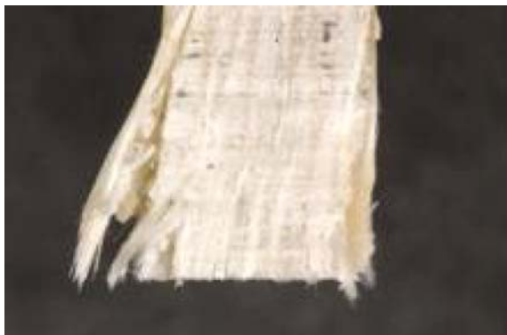
Fig. 27 Cross-section of the plate in test 6 (12.7 mm, 16 kg), showing delamination on the back face
